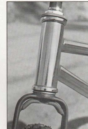
Reinforced Ashtabula forks and steering head of the White Lightning. Notice the space where a gusset usually goes. To find out if this is a boo-boo or not, read the text.
