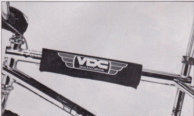
Notice they way the front section is designed. The headtube goes through the top and bottom frame tubes.
