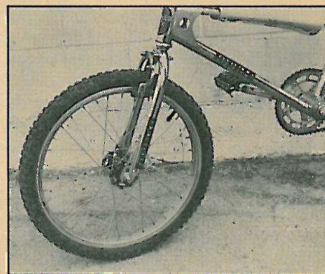
Up front, the TLP has dual head gussets and leading axle forks with a tucked-in axle line. Araya rims, Shimano big hubs and Cheng-Shin rubber make the wheel. Bike uses calipers front and rear.
