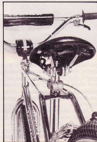
Torkers' distinctive double top tube frame design also appears on the big wheeler.
