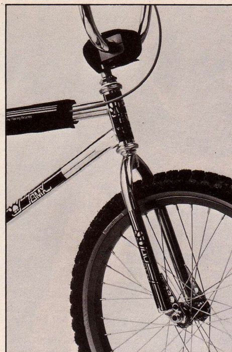
The Team Twenty fork is essentially a Tange TRX unit made in Japan by Tange for JAG. The chrome-plated Trx features a rib-reinforced steering column, oval fork blades and flex-fighting heavy-duty drop outs.
