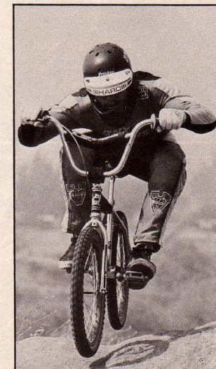
Speed Jumping is easy once you get used to the effect the short rear triangle has on the JAG's balance point.
