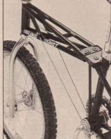
The Sling Shot's "spring plate member," or hinge, is made from a space-age composite called Kevlar, which is the same type of material used in bulletproof vests! High tech.
