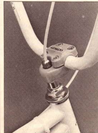
We were only marginally impressed with the Skyway's stem. You have to remove the top piece to tighten the wedge. What's more, the stem didn't clamp the bars as well as expected.
