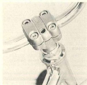
The gooseneck held the bars fine, but wouldn't tighten into the fork adequately.
