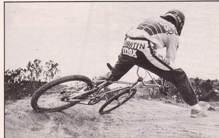
Believe it or not, what you're seeing here is a 17-1/2-inch rear end in action. Not Martin's, you dummy—the Team 24's. The Schwinn Maximizer tires, like most snakebellies, favored the hard pack over the mud and crud we put 'em through during testing.
