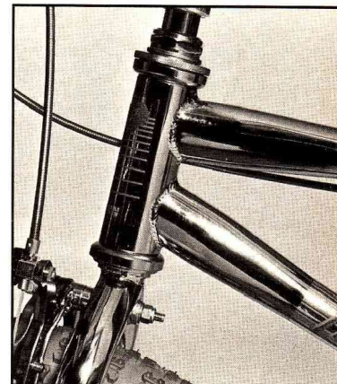
The flared BI-Oval construction at the steering head tube is as slick as ever. Check out the welds — pretty nice, huh?
