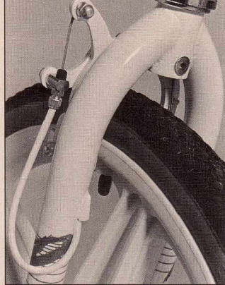
Here's something you wouldn't expect to find on a $200 bike — holes for routing the cable through the fork leg — a Potts Mod accommodation. Installation is a tuff, but the end result is an extremely trick and uncluttered fork leg. Also notice the recessed front brake bolt. Cool idea.
