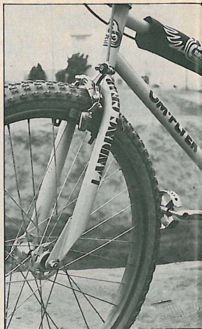
The forks are a larger version of the 20 inch landing gear.
