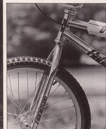
The most welcome change for 1989 is the new forks. As you can tell, they're real straight, which many of you know makes your bike handle real quick. Nice quality and finish, too.
