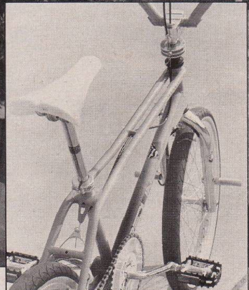
Slender twin top tubes on the 2011 provide enough room for any freestyler, but they're not overdone.
