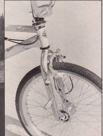
Front-end control on the RL20B is made possible through the six-bolt stem, steep 74-degree head-tube angle and 48-spoke Araya wheels.
