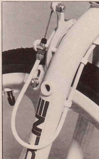
Brazed on cable guides for the Potts Mod and threaded inserts for standing pegs. The inserts go all the way through the fork legs so that when you screw in the pegs you won't have to worry about 'em breakin' off and planting you on your noggin' during a hectic maneuver. Man, is this stuff trick or what? The Pro-Styler runs the new Panaracer Freestyle tires.
