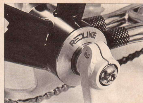
Red Line's new sealed bottom bracket. The bearings are cleverly concealed on the other side of that aluminum shield, so you couldn't get 'em dirty if you tried.
