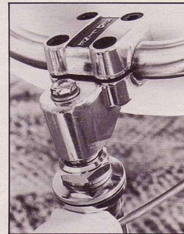
The Super Pro-Line. A cold forged alloy head with chrome-moly stem.
