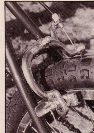
Check the trick tabs on the Dia-Compe calipers. They stop forward whip, make braking more precise.
