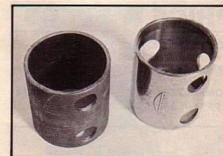
This is TRICK. On the left, your ordinary bottom bracket. On the right, the new Red Line double-butteted and drilled-out jobber. Red Line gave the head tube the same treatment and saved almost a half pound per bike with no apparent loss in strength or rigidity.
