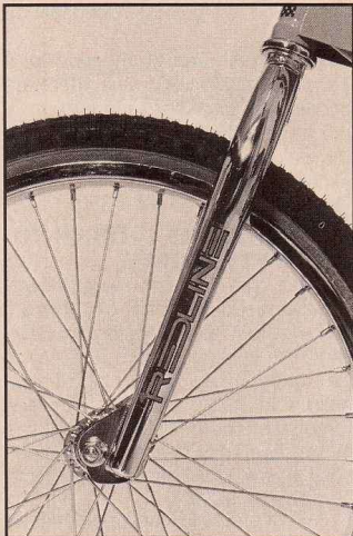
The forks on the 800p have tapered legs, and very stiff front dropouts. Nice.
