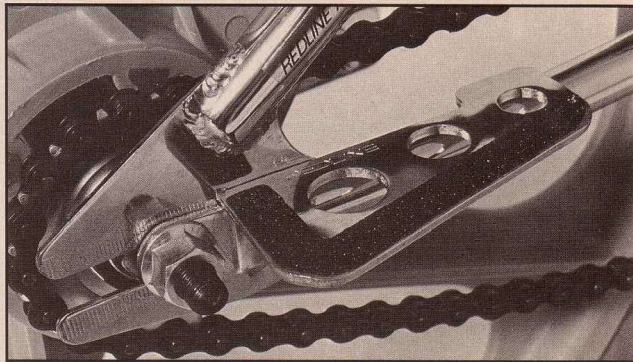
These chain stay standing platforms that come on the RL-20 are probably the neatest units available. They give you gobs of standing area but they're far enough out of the way that you won't shred your ankles while you're street cruising and suchlike.
