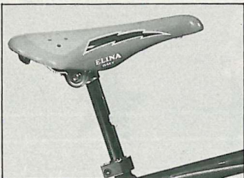
The 24-Inch Race Inc. was equipped with an Elina Seat, Race Inc.'s own seat post and an Xcalibur seat post clamp.
