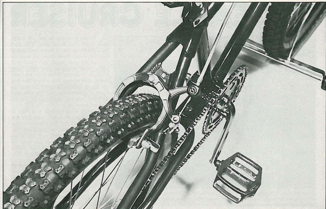
Dia Compe MX1000 brakes were used along with Comp III tires.
