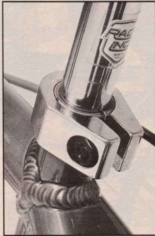
Chrome-moly seat post and aluminum seat post clamp are part of the RA-24 kit.
