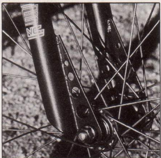
The Race Inc. RF-M leading axle type fork. We found it flex-free for little guys.
