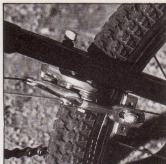
Proper installation of calipers on Race Inc. frames means mounting the unit upside down as shown.
