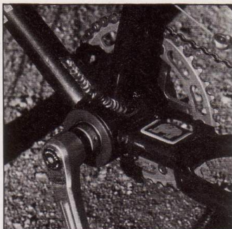
The large even fillet at the joints indicates good penetration at the welds.
