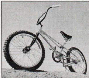
This is class machinery. Check the double top-tube frame construction. Low profile of the R&R RESULTS IN A LOW CENTER OF GRAVITY AND THE LOW C/G provides for amazing handling characteristics. Seat is definitely not moto.
