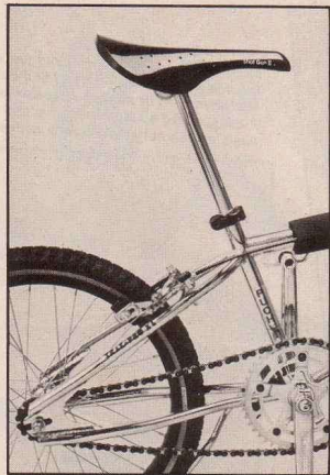
Not unlike Speed Unlimited's Thruster-style rear end, the Puch features unique "trapped"-style rear dropouts and gusseting at both the seat stay/seat tube junction and the chain stay/crank hanger juncture. To sum it all up in one word: strong.
