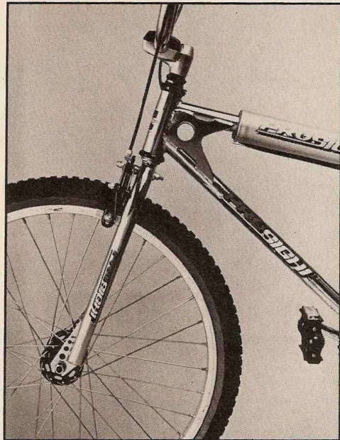
The Prosight features Tange's slightly ovalized TRX chrome-moly forks, 1-1/8" top and Dia-Compe 890 callipers front and rear, SR stem, Takagi cro-mo cranks and KKT pedals—winners circle stuff.
