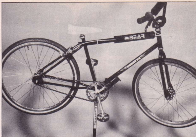
This bike came equipped with (as built by Dave's Bike Shop, Riverside): Prodyne cruiser frame, Prodyne handlebars, Prodyne seatpost clamp, Bear components (bottom bracket, pedals, headset, gooseneck), Haro lever, Uni-seat, DuraAce cranks, Dia-Compe brakes, Sunshine hubs, Araya 26-inch wheels with Mitsubishi stadium tires.
