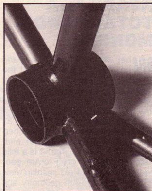
A double gusset bolsters the chain stays.
