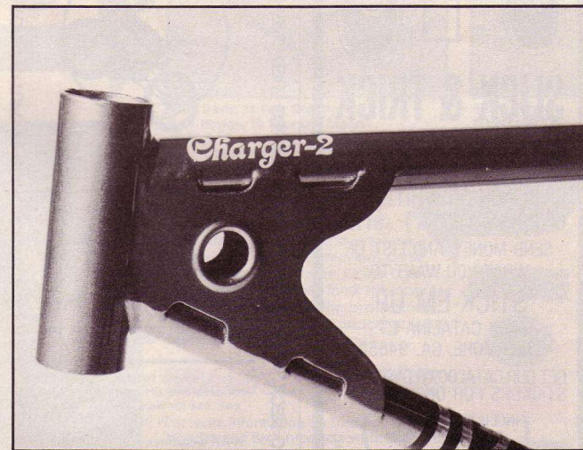
Space welded gussets fortify the steering head juncture. Ignore the Charger-2 decal. It should read Charger.
