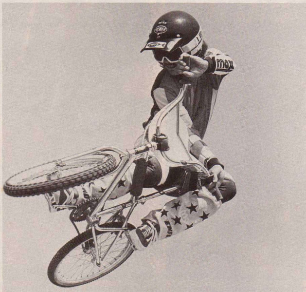
The rear stay width allows for the use of wider, longer-wearing, 2.125" tires. Haselhorst runs a 1.75" rear and a 2.125" front.
