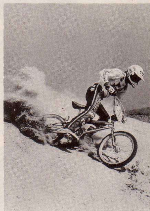
The rear stay width allows for the use of wider, longer-wearing, 2.125" tires. Haselhorst runs a 1.75" rear and a 2.125" front.
