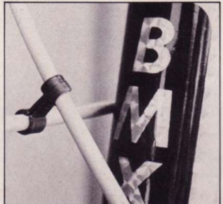
This is trick! It's a little clamp-jobber that holds the brake cables where they cross. What kind of mind invents stuff like this?
