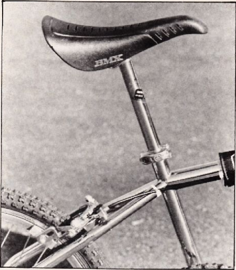
The seating was first class all the way. Eric uses a special 14-inch chromoly post on his personal scooter, but our tester (which Eric rode for most of our photos) came with a 12-incher. We'd like to see the longer one become standard.
