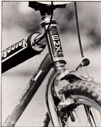
Dia-Compe MX-1000s are standard, front and rear. Note the typical BMX Products attention to detail in the graphics and craftsmanship.
