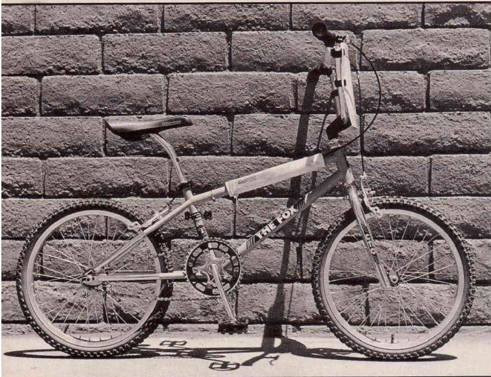
The Fox Special Edition held up great with the exception of the left pedal. Kirk wasted the nylon end after an extremely harsh landing at Lucky’s in Huntington Beach. No other tweakage reported. To clear up a couple of things, the bike doesn’t come with the number plate or Flite’s Pad-Lock pads (we put ‘em on for the test, but couldn’t get ‘em off without the key, which we’d left at the office). Also, disregard the U.F.O. decal on the forks; the new Special Edition logos weren’t ready yet for our test vehicle.
