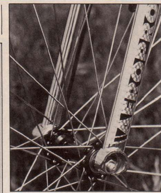
The AeroPro's elliptical fork legs feature RRS-like dropouts. The overall finish quality, decals, etc., were pretty well received by all.
