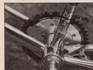
Clean bottom-bracket action. A simple chain stay gusset keeps rear-end whip to a minimum, while chromoly cranks, power disc and YST chain put the power to the ground.
