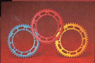
"Dura Ace", "600EX" and "UltraDyna" chainrings can all be used with the Tourney.
