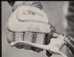
The brake lever supplied is unbent and works almost not at all. To stop it from jamming your fingers, it must be bent.
