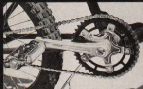
Some very zoot equipment: KKT chrome-moly pedals, Takagi Tourney alloy 6 1/4 inch cranks, and a Takagi alloy sprocket.
