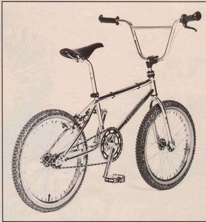
The '83 Kuwahara Lazer Lite. Gussets are gone, CG is higher, lots of trick stuff has been added.
