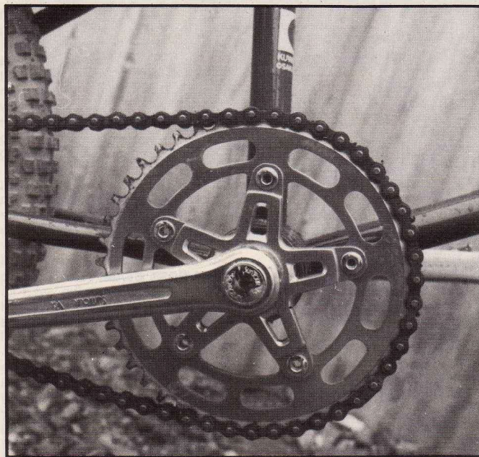
Suntour three-piece cranks a little wimpy but get the job done.
