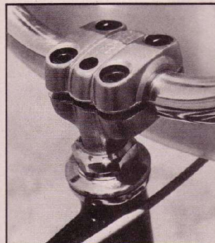
The Sun Tour forged aluminum gooseneck is cosmo equipment . . . but better suited for smaller guys' bikes than for the full size Kuwahara.
