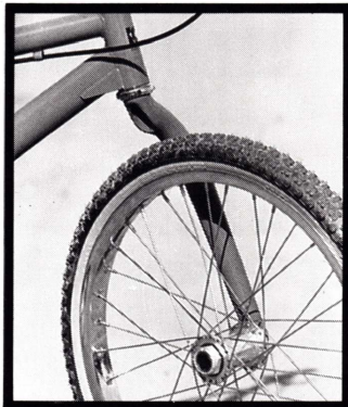
Is this the incredible disappearing bike or a product of modern technology? Linn Kastan created this beefy Uni-Blade (or Strut) to be stiffer and lighter than the conventional fork.
