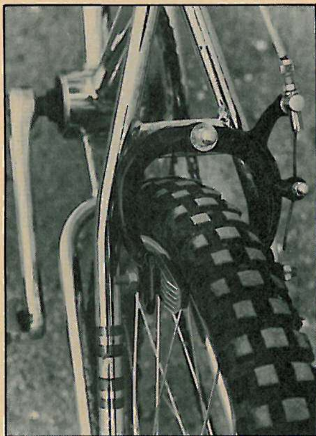
An apparently non-standard piece of equipment that we found was the Schwinn-approved side-pull caliper. Seen in the back is a definitely stock Shimano Dura-Ace alloy crank, with SunTour pedals.
