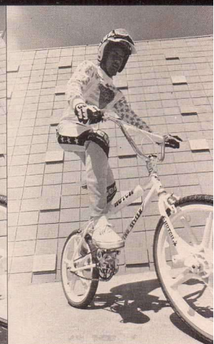
The chain stay platforms are a little far forward, but they work fine. The dropout/coaster brake bracket is sano. Check out the new Hutch mags.
