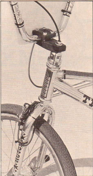
Although our test bike came with a conventional Hutch stem, Woody's personal trickster has a Power Products "Rob Modification" cable routing arrangement. It's similar to the famous Poits Modification. Note also the distinctive tubular gusset on the Trick Star. Trick indeed.
