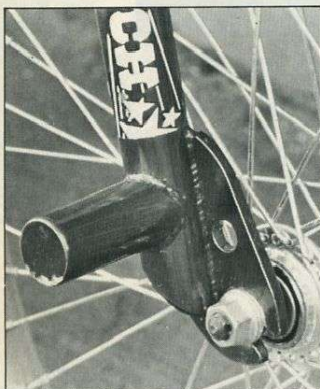
The Hutch fork pegs. Even though they can stand in the way of pulling off some tricks (Miami hoppers in particular), they are placed in a comfortable spot and are large enough to accommodate Bigfoot!
