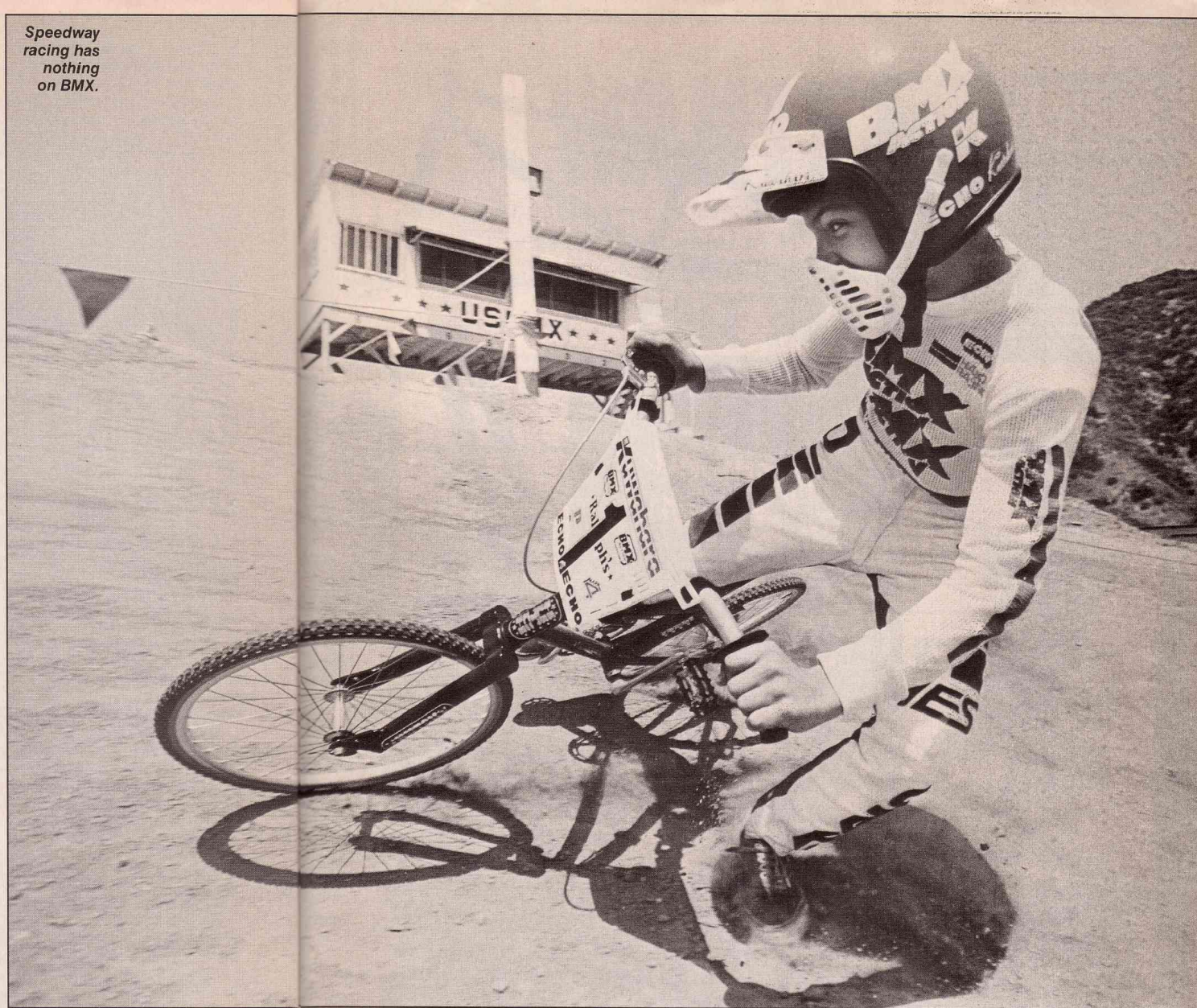
The Hutch mini stems come in three sizes—a 1 inch reach, a 1 1/2 incher, and this one here—the 2 inch reach. Also shown is the magnesium headset, which has a teflon ring instead of ball bearings. Not quite the smoothest thing we've ever used.
