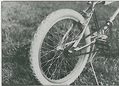
The light Araya or Ukai box-style anodized alloy rims are a trick racing feature. Cheng-Shin colored gumwall tires round out the package.
