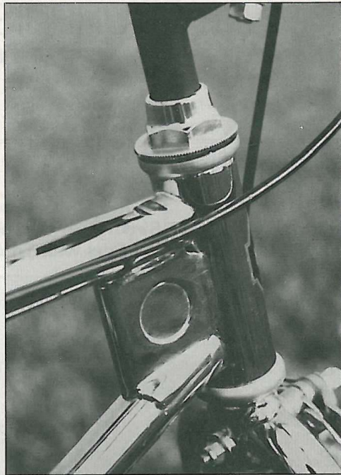
Head tube angle is 71°.
