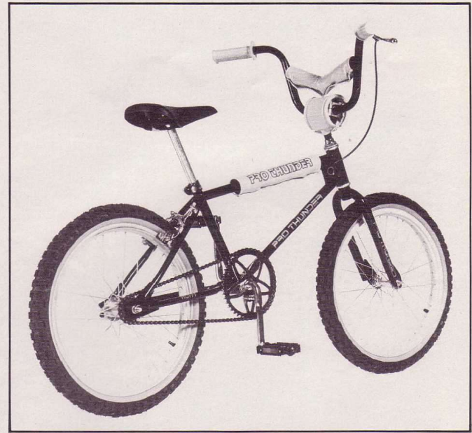
This is the Huffy in half-race trim. Which means we removed everything that wasn't absolutely necessary for racing. We didn't replace any components at this point. The weight went down to just under 30 pounds. This would be a pretty fair beginner's race bike.
