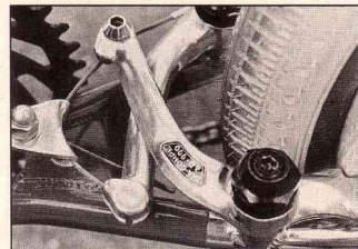
Haro tricked everyone and mounted the 990s on top of the chainstays. No they don't really get in the way as much as you're thinking they do.
