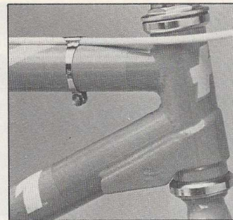
A wrap-around front gusset, along with chevrons stamped into the steel, tell you the RS3 is made by Haro.
