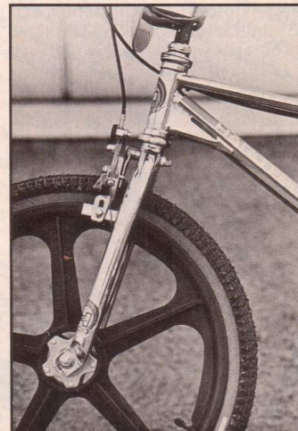
Some of the beefiest forks in the biz combined with a specially machined head tube and wedge gusset add to the Freestyler's unique looks and superior strength.
