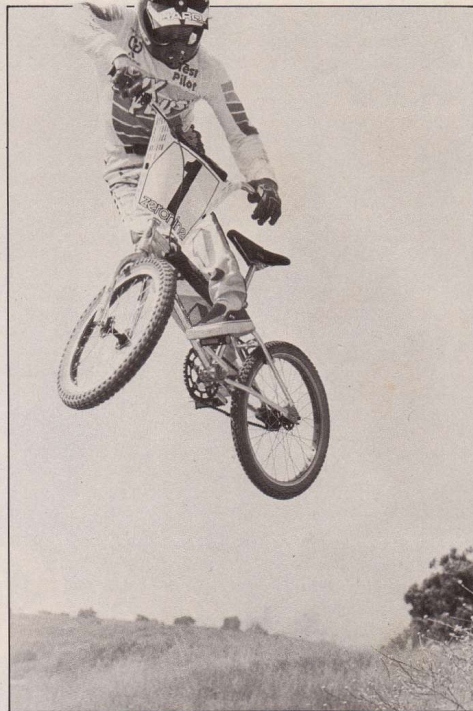
The proven 44/16 gearing and SR's super-dependable 175mm chromoly cranks make building up a head of steam and landing lofty leaps like this no prob at all.
